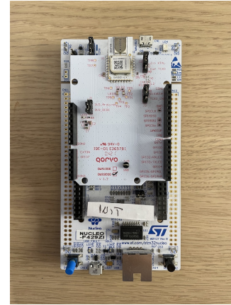
Figure 1: Shows a NUCLEO-F429ZI with the DWM3000EVB attached.
